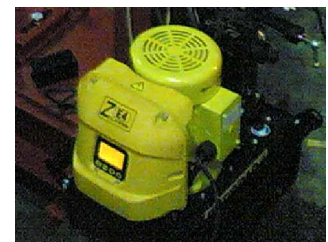
Hydraulic system for force generation and adjustment
