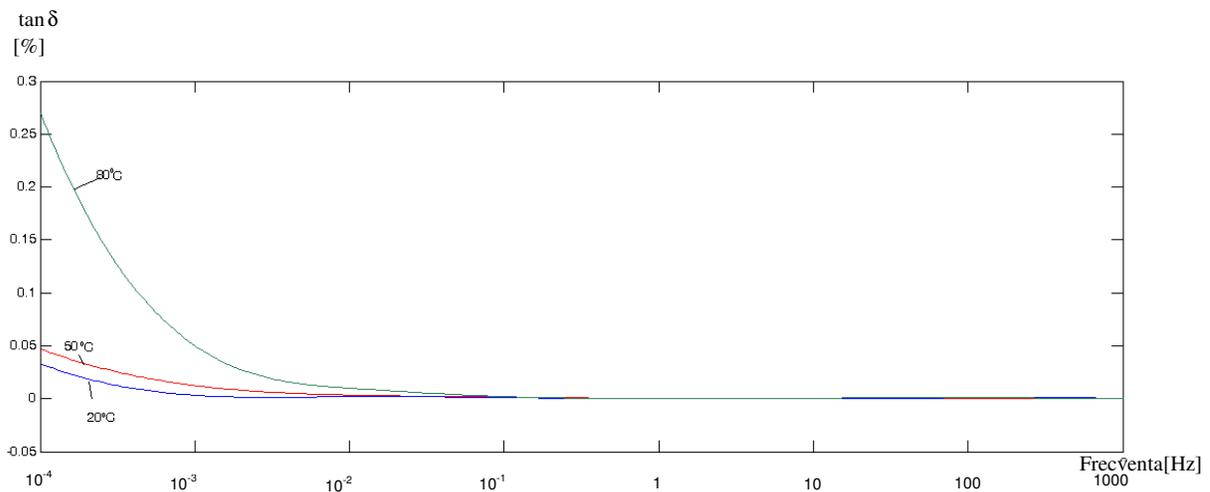
Fig.2. Dielectric response versus temperature for a transformerboard specimen impregnated with oil with a moisture of 1%
