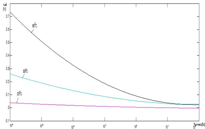
Fig.4 Dielectric loss factor versus frequency for a test specimen with a moisture of 1%
