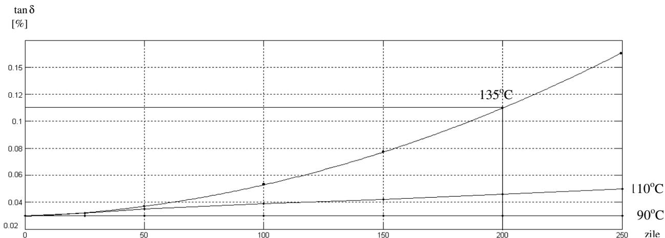
Fig.6. Loss factor dependence upon the ageing. Measurement performed at a temperature of 50°C
