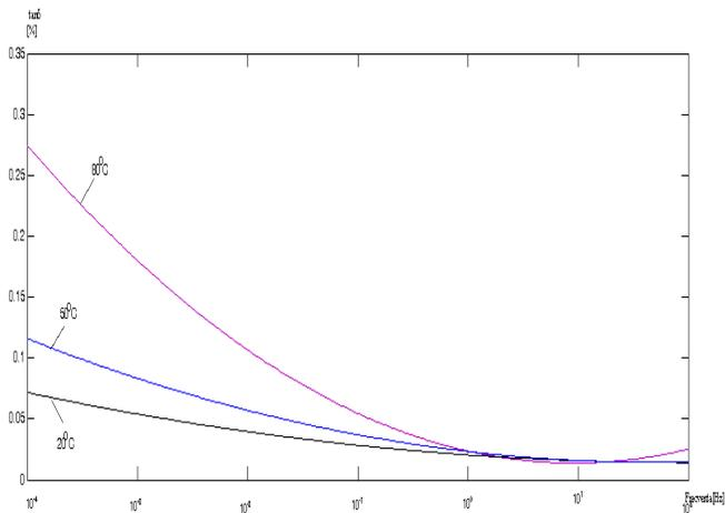
Fig.3 Dielectric loss factor versus frequency for a test specimen with a moisture of 2%
