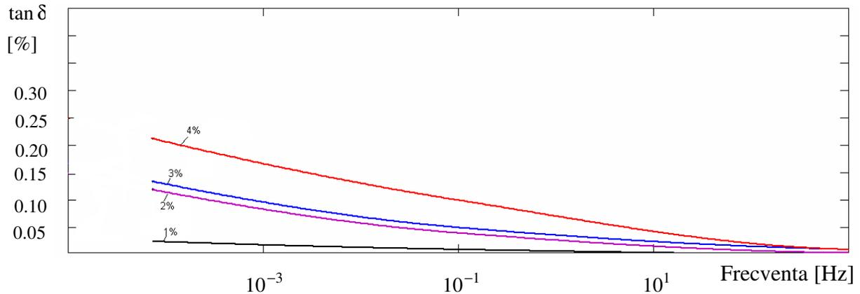
Fig.1. Mean dielectric response of transformerboard – oil insulation system with different moistures
