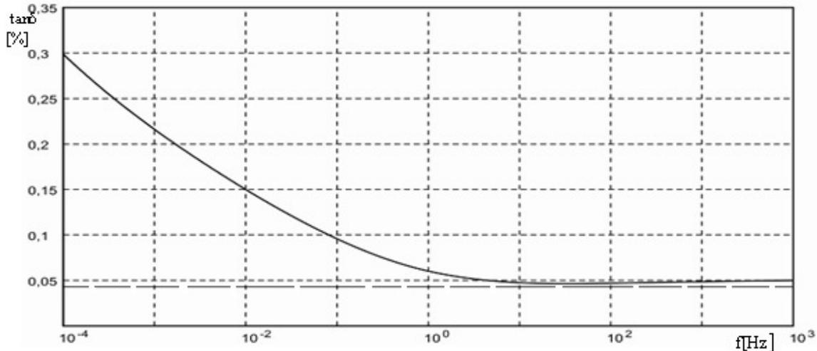
Fig. 7. Comparison of the frequency response of transformerboard-oil system for aged and non-aged cases; — insulating system aged for 250 days at a temperature of 90°C --- non-aged insulating system; Systems moisture: 0,5%; Measuring temperature: 50°C
