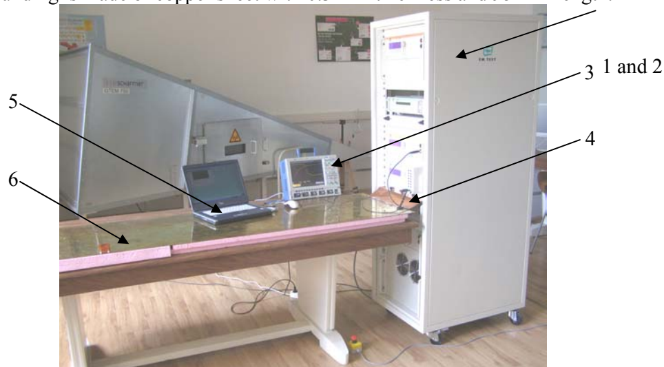
Fig. 15 Test set-up for immunity to conducted transient disturbances
