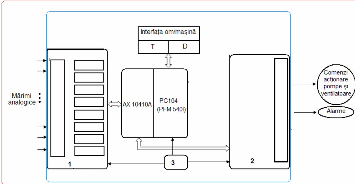
*Fig. 1. Block diagram of the monitoring equipment*
