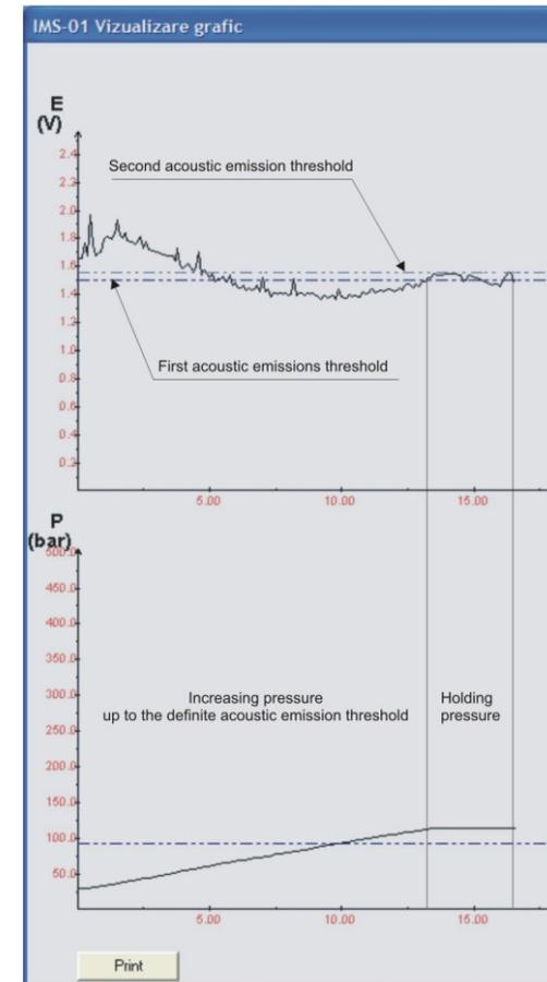
The method for crimping the fitting on the composite insulator rod using AE and crimping pressure monitoring provides:
